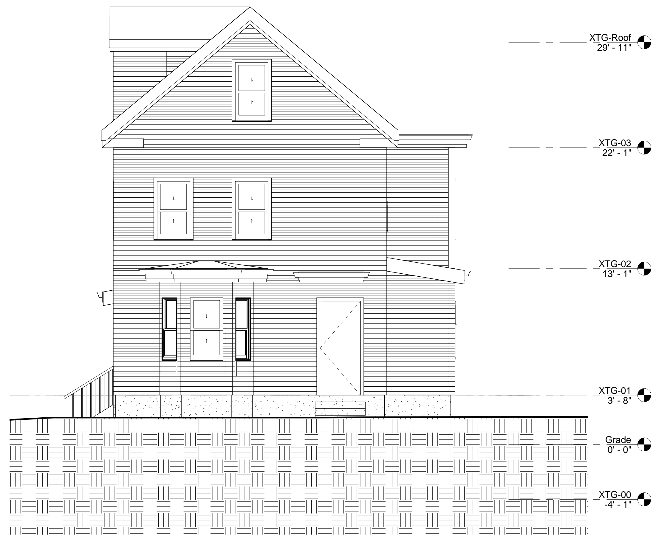
① EXISTING EAST ELEVATION 1/4" = 1'-0"
